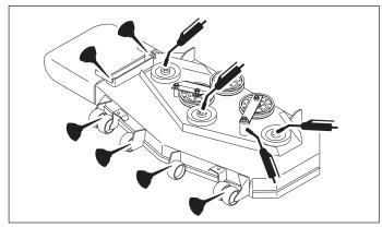
Figure 15. Deck Lubrication
